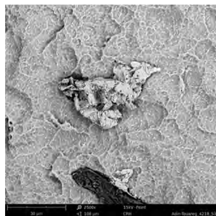
27 | Same implant surface (Adin Touareg): bright chromium-nickel-iron particle, dark aluminium oxide particle (x2,500).
